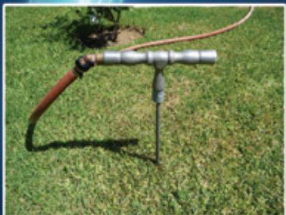
Use the 3 / 8 Metal Pipe when finding the Drain Pipe
